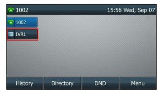
Press the line key (IVR1) to perform the macro definition of the action IVR1 (10086\$Tinvite\$\$Cwaitconnect\$\$P5N4\$\$Tdtmf\$\$Cpause2\$4\$Tdtmf\$\$Cpause1\$2\$Tdtmf\$).
